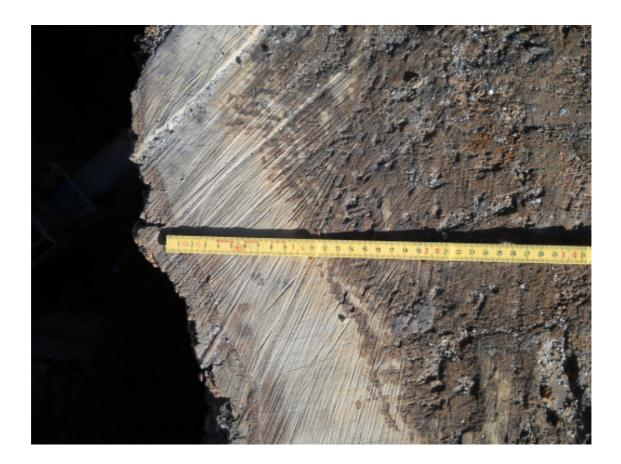
Picture 5 The thickness of sound healthy wood is in parts less than 10 cm
