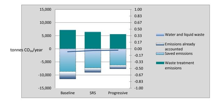
Figure 5. Summary of waste emission reductions due to waste measures
