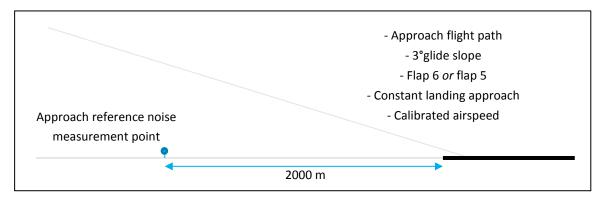
*Figure 1: Setup for analysis of approach noise level reduction. The landing approach calibrated airspeed (as defined in ref. 10) is based on the selected flap setting and the modelled landing weight*
