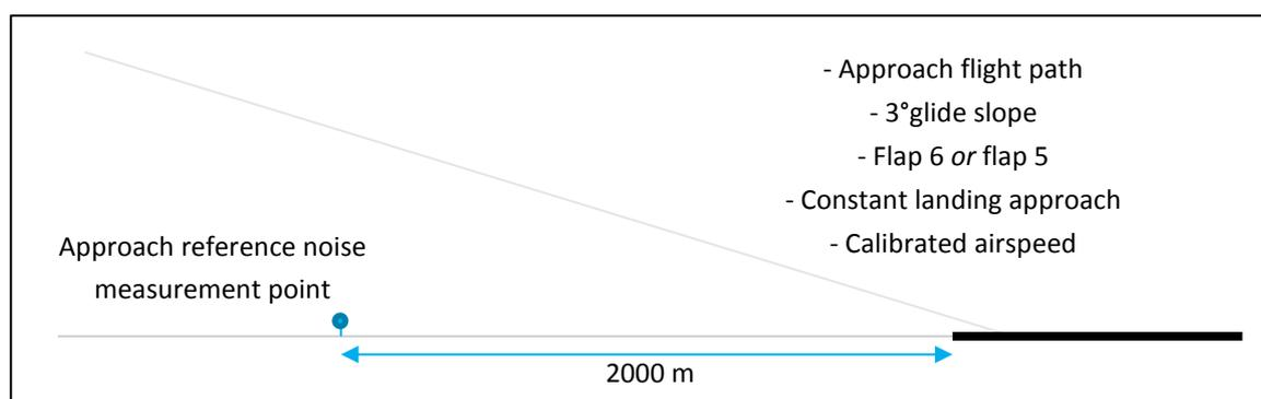
Figure 1: Setup for analysis of approach noise level reduction. The landing approach calibrated airspeed (as defined in ref. 10) is based on the selected flap setting and the modelled landing weight
