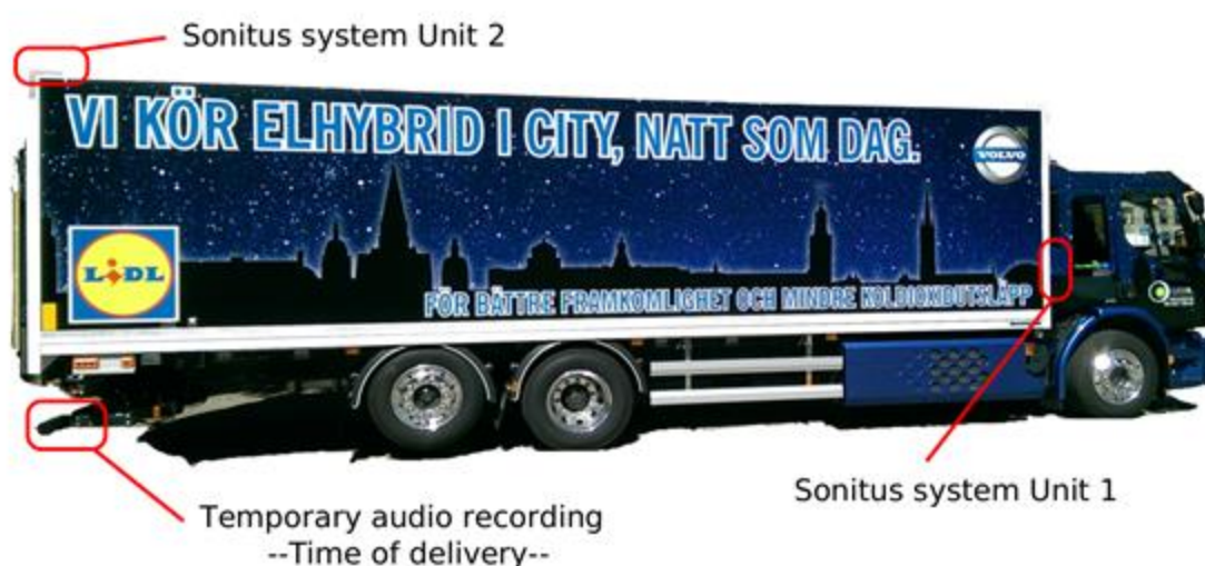
Figure 3: Noise monitoring setup illustrated on the Volvo truck: back and front
