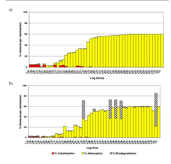
Figure 7: Percentage of each removal mechanism during primary sedimentation stage according the Byrns (a) and the STPWIN (b) models
