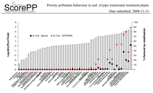
Figure 9: Percentage removal via volatilization during secondary sedimentation stage
