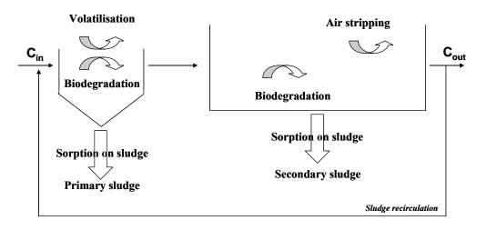
Figure 2: Major pollutant removal pathways in conventional activated sludge waste water treatment
