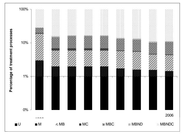
Figure 1. Processes applied in Danish wastewater treatment plants
