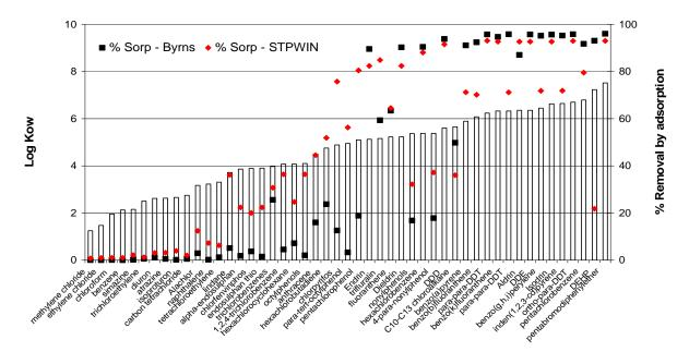
Figure 10: Percentage removal via sorption during secondary sedimentation stage
