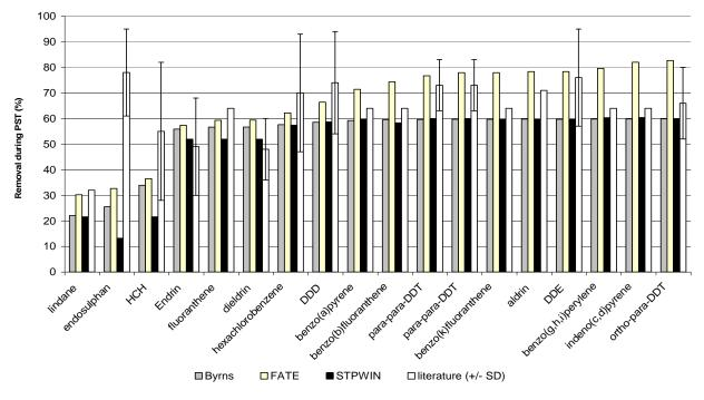
Figure 3: Model predictions compared with literature data for PP removal during the primary sedimentation stage
